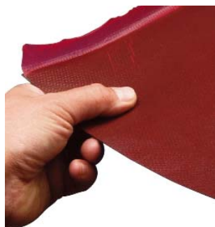
Intumescent material in sheet form
